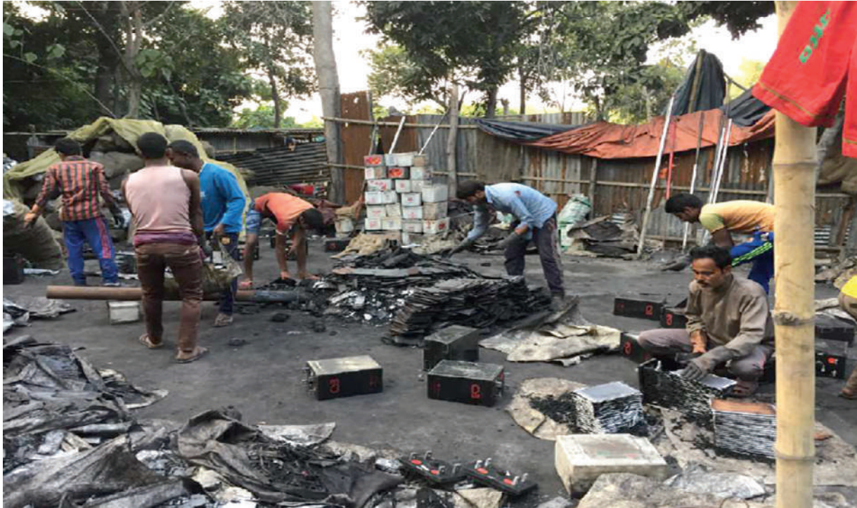
Figure 27: Used Lead Acid Battery Informal Recycling Factory
