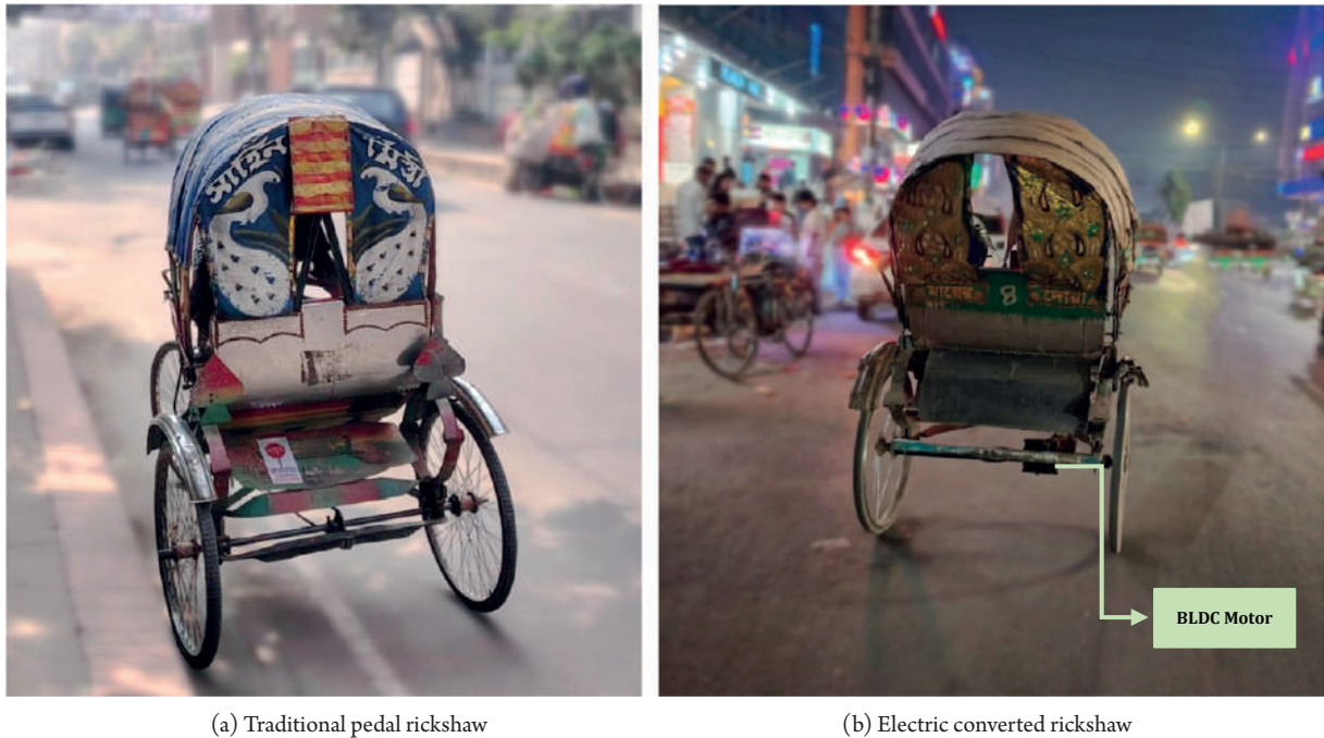
Figure 11: Pedal to Electric Rickshaw Conversion
